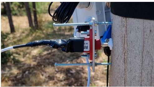
c) The Generic Digital Dendrometer, attached to the eucalypt.
