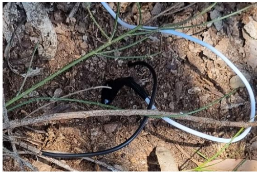
a) The 18B20 Temperature sensor and Capacitive Soil Moisture Sensor V1.2 Placed 5cm deep into the soil.
