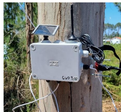
b) GWD9 strapped to a eucalypt in Leiria, Portugal. Equipped with a solar panel and a 3dBi antenna.
