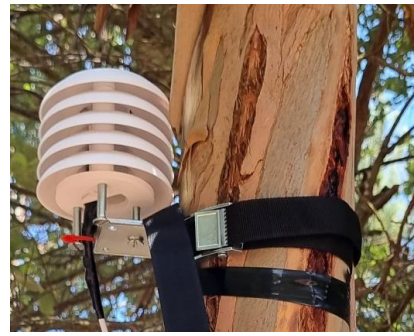
b) The DHT22 enclosed by a 3D-printed Stevenson screen, strapped as close as possible to the start of the canopy.
